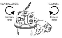
B. Sensor is picking up mirror or highly reflective wall or surface in front of fixture. Install Optima Plus<sup>®</sup> slightly "off-center" (2 to 5 degrees) to eliminate direct reflection off of mirror or opposite wall or surface.
