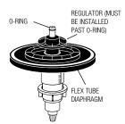
The flush volume of the flex tube diaphragm kit is controlled by the regulator. Regulators are identified by color. Some flex tube diaphragm kits are supplied with multiple regulators. The installer must make sure the proper regulator is used when installing the flex tube diaphragm kit.
