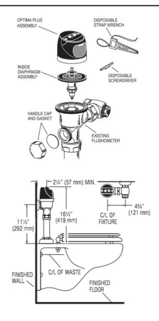
When installing the Optima Plus in a handicap stall: Per the ADA Guidelines (section 604.9.4) it is recommended that the grab bars be split or shifted to the wide side of the stall.
