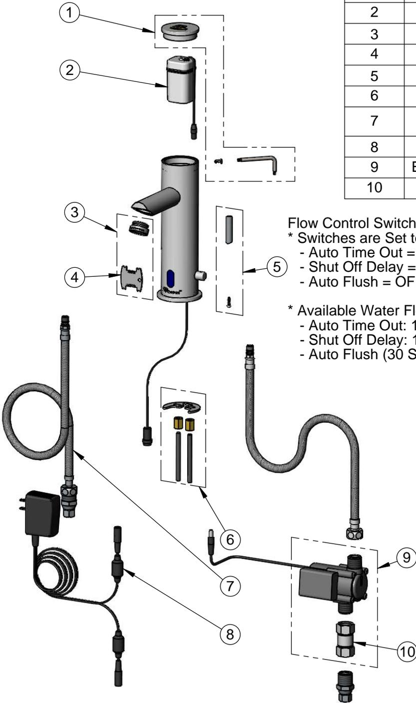
Flow Control Switches are Located Beneath the Cap.
