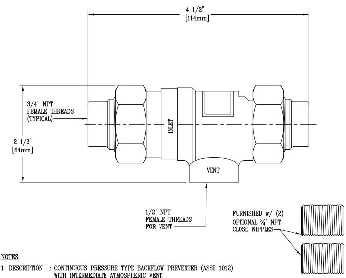
2. CONSTRUCTION: CHROME PLATED BRASS BODY WITH STAINLESS STEEL WORKING PARTS, INTEGRAL STRAINER, & DURABLE RUBBER DISCS. WEIGHT = 1.8 LBS.
