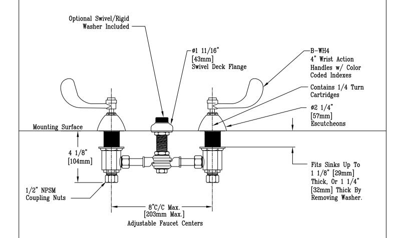
Note: Rough-In Required: ø1"[25mm] For Center Shank ø1 1/2" [38mm] For Hot/Cold Side Bodies [1-1/4" [32mm] Minimum]
