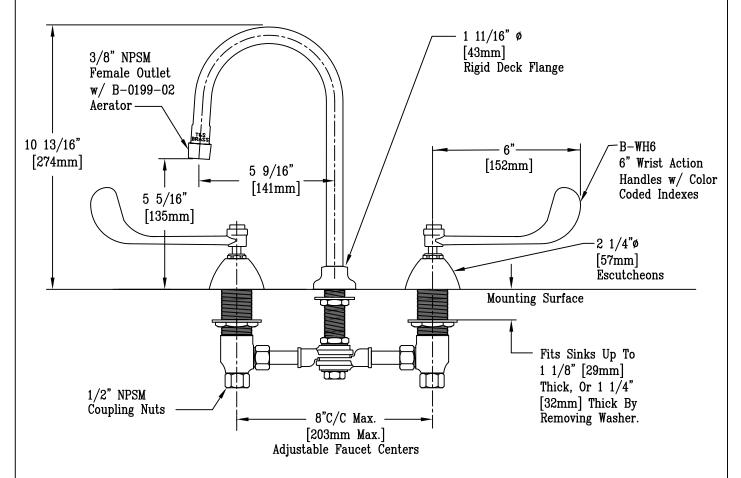
Hot & Cold Center Sections Can be at Angle
