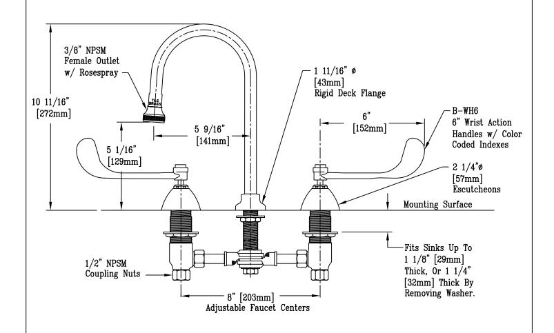
Note: Rough-in Required: \$\phi7/8\$ for Center Shank \$\phi1 1/4\$ for Hot/Cold Side Bodies
