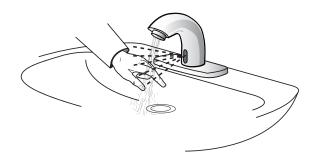
1. Place hands under faucet. Solenoid valve should "click," LED in sensor window should blink once and water should flow from the spout.
