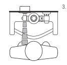
3. When the user steps away from the OPTIMA® Sensor, the circuit immediately initiates an electrical "onetime" signal that operates the Solenoid. This initiates the flushing cycle to flush the fixture. The Circuit then automatically resets and is ready for the next user.
