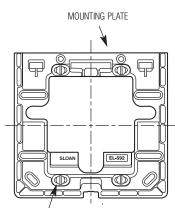
4" (102 mm) SQ. x 2-1/2" (64 mm) DEEP OUTLET BOX — APPLETON ELECT. #4SD1 OR EQUAL (BY CONTRACTOR)
