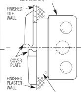
4" (102 mm) SQ. BOX DEVICE COVER (PLASTER RING) 3/4" (19 mm) HIGH — APPLETON FLECT. #8470 OR EQUAL (BY CONTRACTOR)
