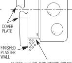
4" (102 mm) SQ. BOX DEVICE COVER (PLASTER RING) 3/4" (19 mm) HIGH — APPLETON ELECT. #8470 OR EQUAL (BY CONTRACTOR)
