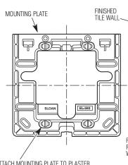
ATTACH MOUNTING PLATE TO PLASTER RING USING FOUR (4) SCREWS (SUPPLIED) 4" (102 mm) SQ. x 2-1/2" (64 mm) DEEP OUTLET BOX — APPLETON ELECT. #4SD1 OR EQUAL (BY CONTRACTOR)
